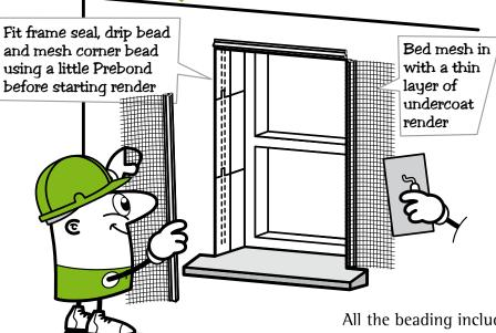
All the beading including the clip on drip bead should be fitted before rendering takes place
